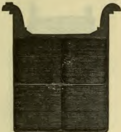
FIG. 426. —"Unformed" Plate of One Pattern of "Gould" Storage Cell. The particular plate shown has total outside dimensions of 6x6 inches. The clear outline of the grooves indicates absence of oxides, due to action of "forming" solutions, or charging current.
